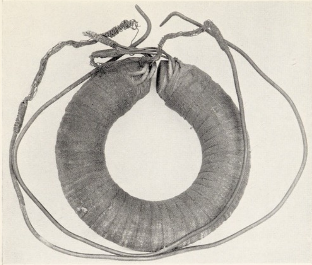
FARADAY'S GREAT RING ELECTRO-MAGNET. From a photograph by the Science Museum, South Kensington.
