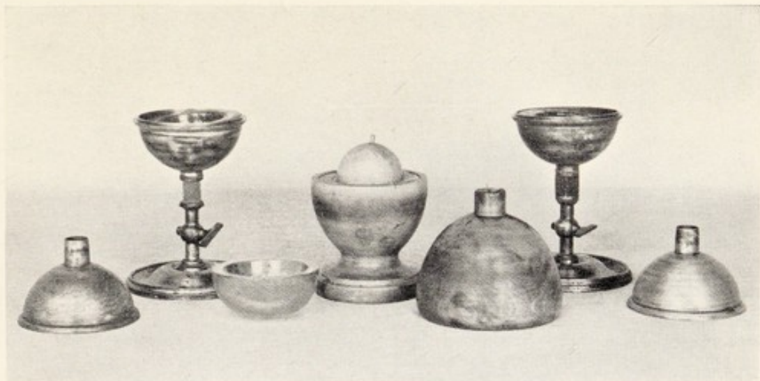
FARADAY'S SPECIFIC INDUCTIVE CAPACITY APPARATUS. From a photograph by the Science Museum, South Kensington.
