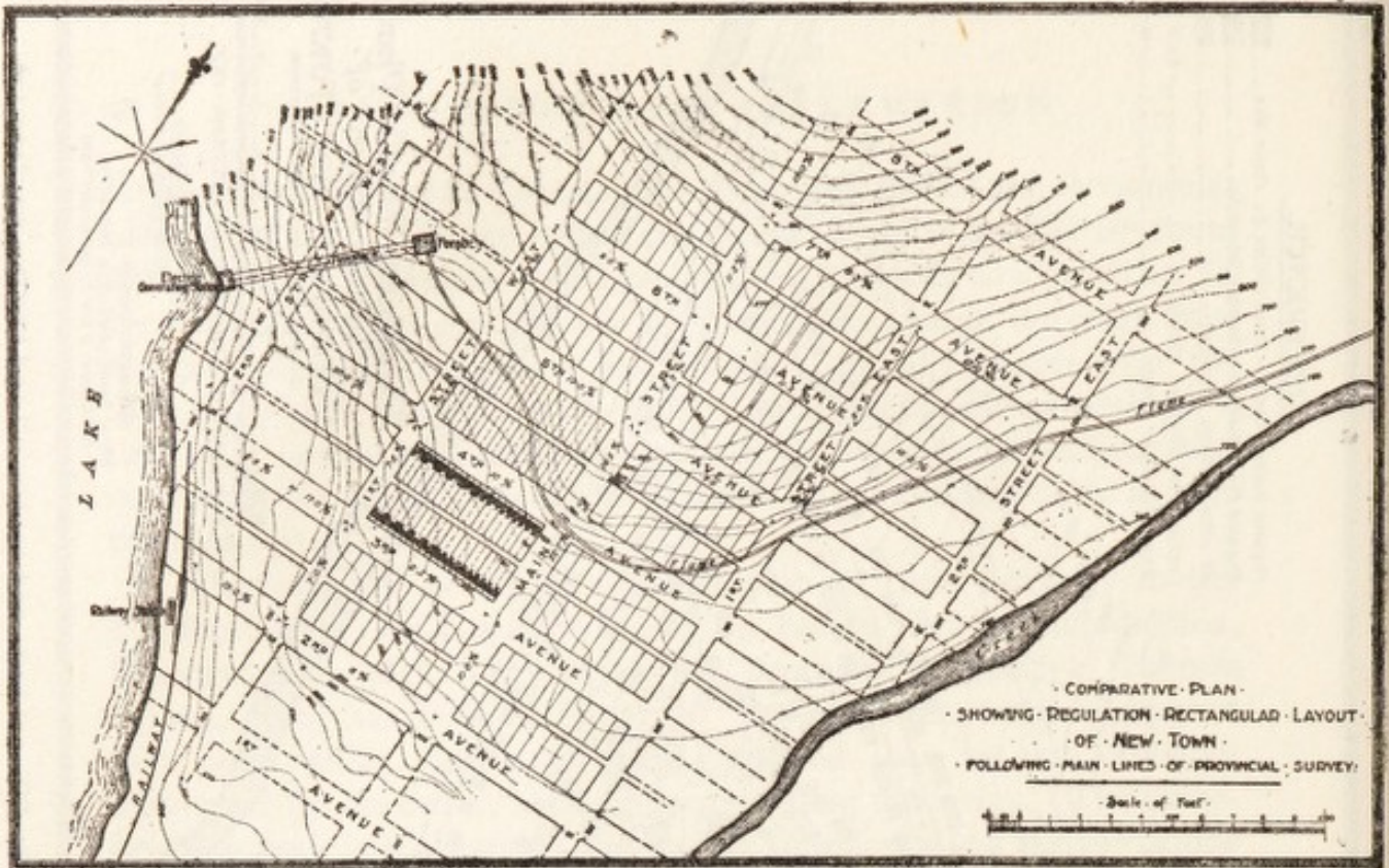
Rectangular Plan of Area included in Figure 19, designed to secure conformity with provincial survey, but no object of convenience or economy of development. See page 67.
