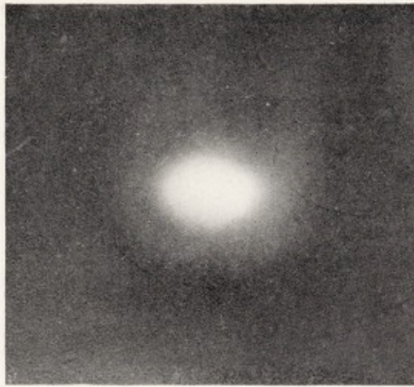
FIG. 6.—PINHOLE PHOTOGRAPH OF SPOT ON TARGET WHERE THE X RAYS ORIGINATE —FRONT VIEW.
