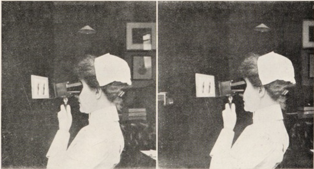
FIG. 19.—METHOD OF VIEWING WITH THE BREWSTER OR LENTICULAR STEREOSCOPE.
