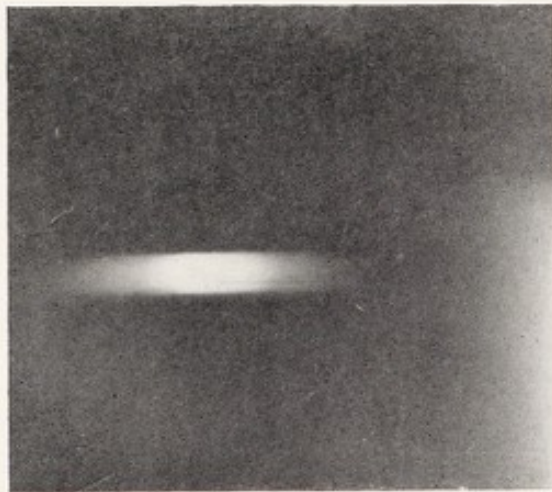
FIG. 7.—END-ON VIEW OF X-RAY PRODUCING SURFACE ON ANODE OR TARGET OF A TUBE.
