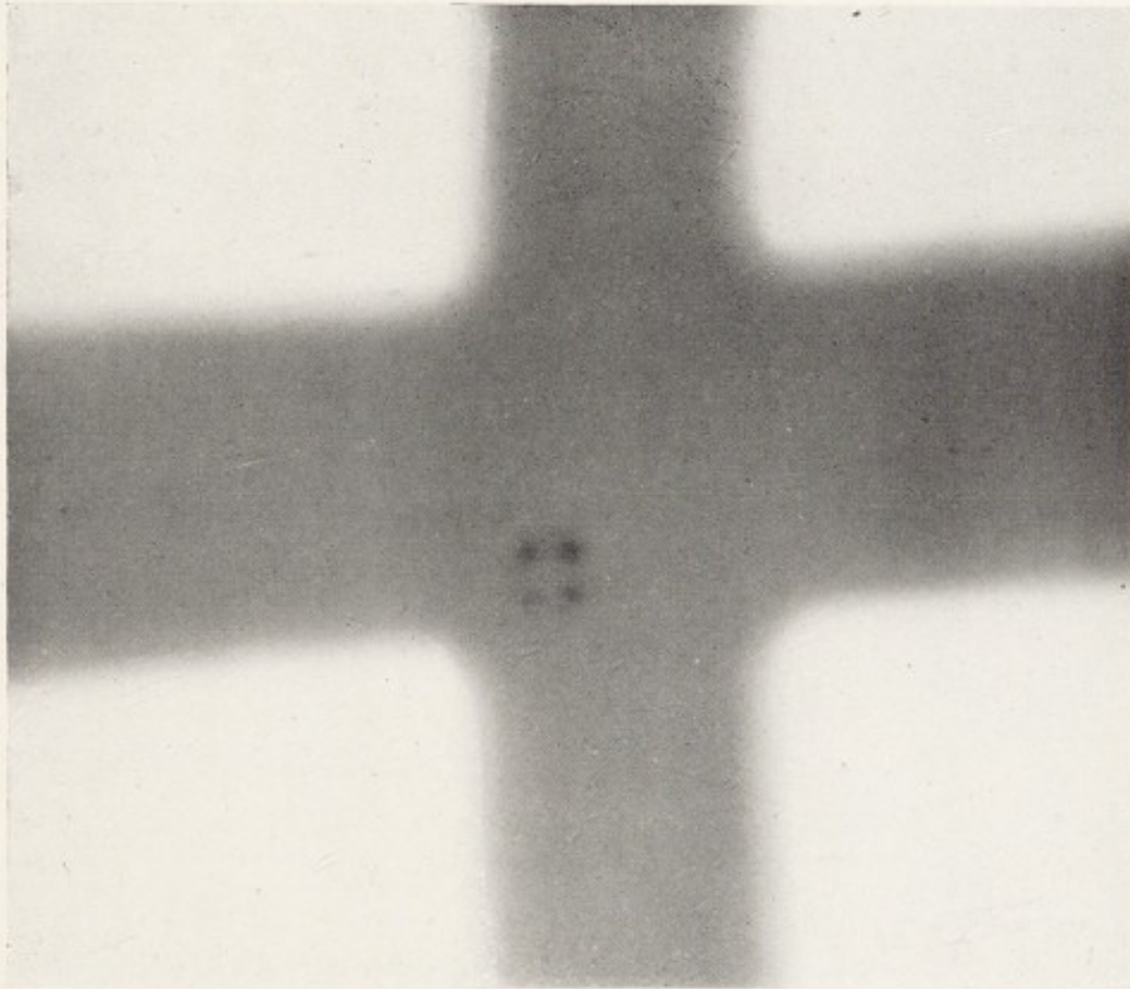
FIG. 12.—FOUR IMAGES OF A METALLIC OBJECT SEEN WITHIN THE INTERSECTION OF A CROSS OF LEAD WHICH HAD BEEN PLACED IN FRONT OF THE TUBE.
