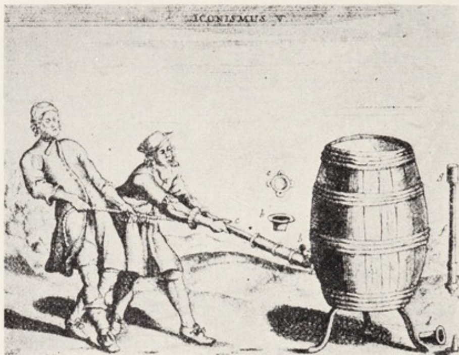
FIG. 4. Von Guericke's experiment of using a water pump to draw water from a full cask in the attempt to create a vacuum.
