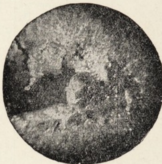
FIG. 19.—Photomicrograph of a platinised nickel anticathode fused by a discharge.
