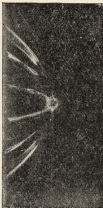
FIG. 11.—Photograph obtained by J. J. Thomson of parabolic loci of positive particles subjected to magnetic and electric fields at right angles to each other. The different traces represent different substances. In the figure, the magnetic deflections are vertical. The magnetic field was reversed half-way through the exposure, so that both halves of each parabola are recorded.
