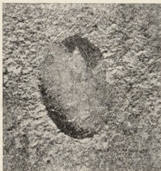
FIG. 23.—Photomicrograph of fused focus-spot in a tantalum anticathode.
