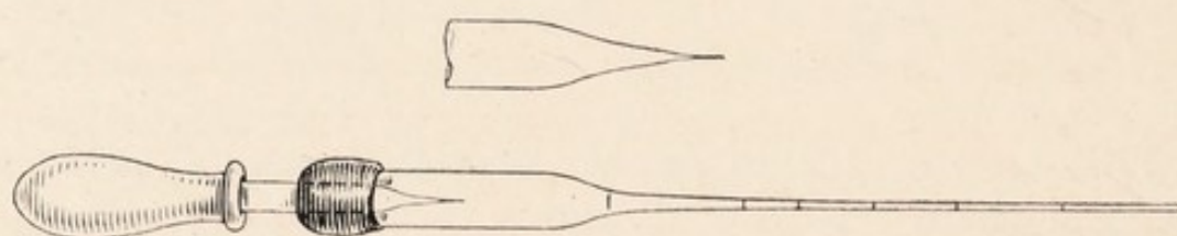
FIG. 8.—" Throttled " pipette. The upper figure shows the fine point of the " throttle."
