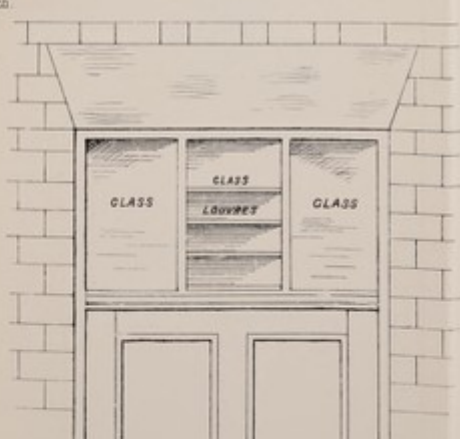
ELEVATION OF FANLIGHT OF FRONT DOOR SHEWING GLASS LOUVRES FOR VENTILATION.
