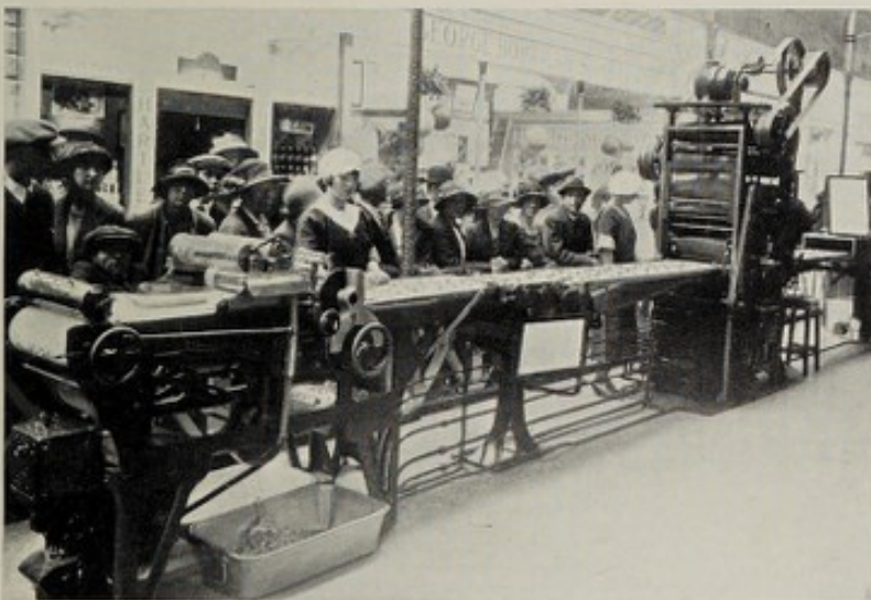
FIG. 173.—A CHOCOLATE-COVERING MACHINE IN CARSON'S EXHIBIT, WEMBLEY, 1924.
