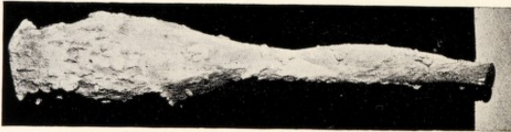
FIG. 1.—POINTED (SERVICE) BULLET. ·22 CALIBRE. CAST OF EFFECT IN CLAY.
