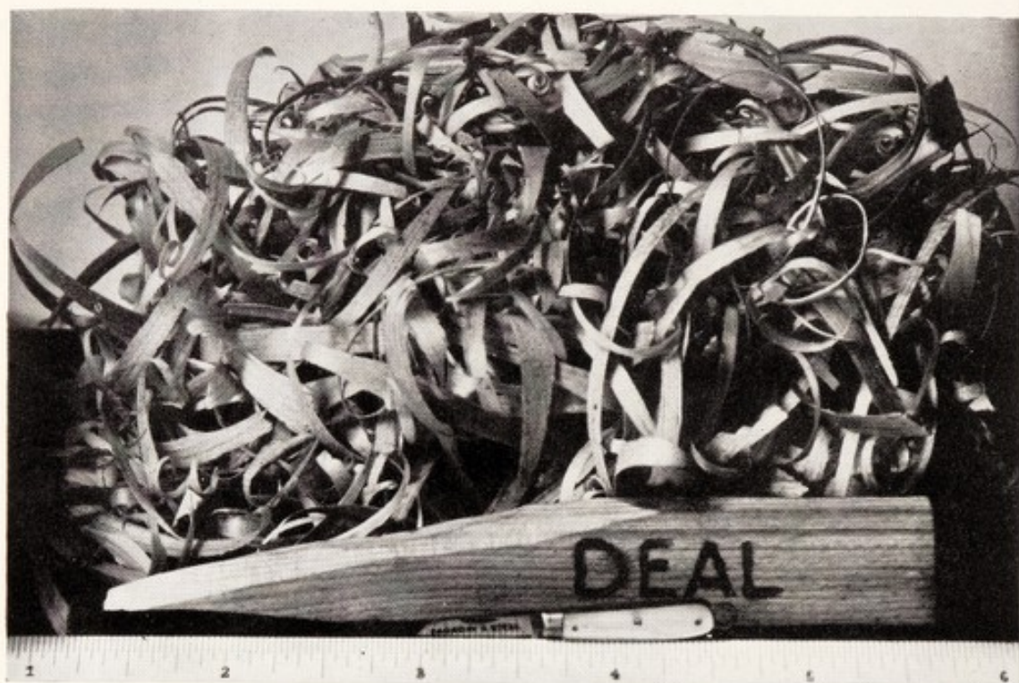
SHAVINGS CUT BY THE MINIATURE KNIFE ILLUSTRATED, MADE OF FARADAY'S STEEL. The blade of this knife weighs only one-hundredth of an ounce, the complete knife weighing one-twentieth of an ounce. The shavings, cut from a block of deal, weigh about eighty times as much as the blade itself. After producing these shavings the blade was still in excellent condition.
