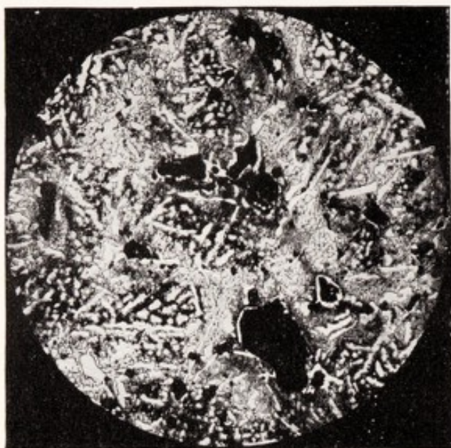
PM. 7. (X 200.) 68/F. 2. C 1.75. S 1.76 %. POLISHED AND ETCHED.
