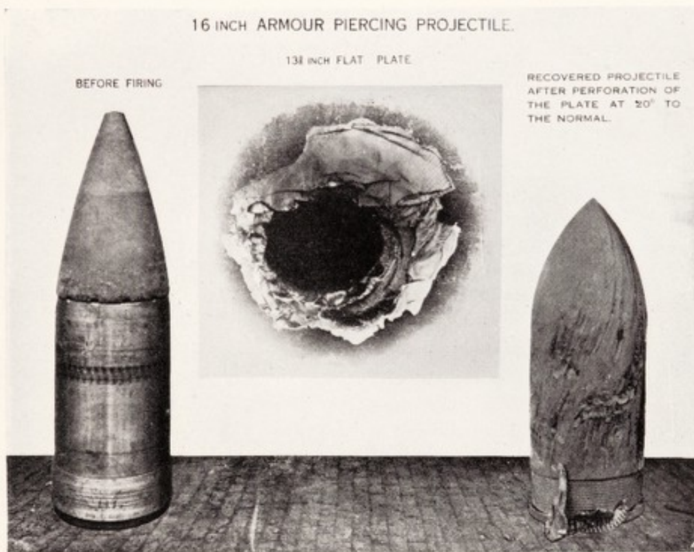
HARD-FACED ARMOUR PLATE 14 IN. IN THICKNESS, INCLINED 20°, PERFORATED BY A 16 IN. CAPPED ARMOUR-PIERCING PROJECTILE IN .00314 OF A SECOND.
