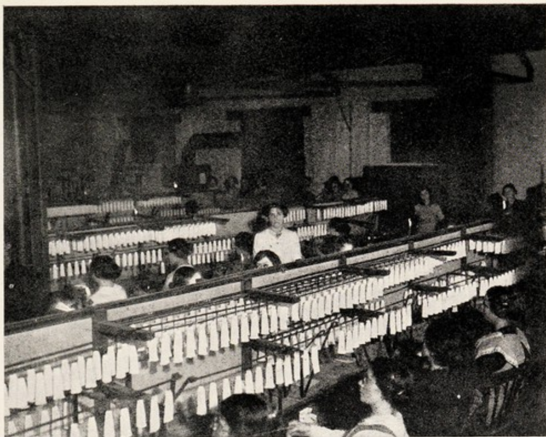
FIG. 73.—VOLKER LIGHTING CORPORATION, LTD. SEASONING UPRIGHT MANTLES.
