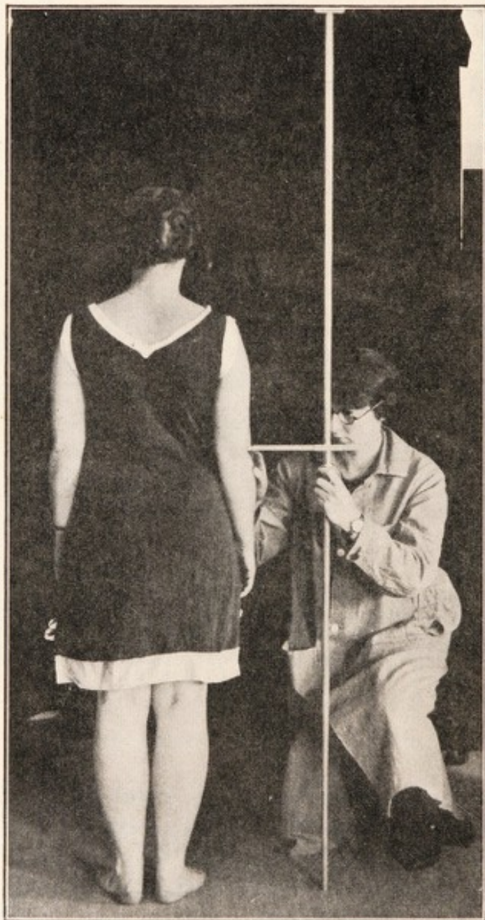
FIG. 5.—Anthropometer, being used for ascertaining heights from floor.
