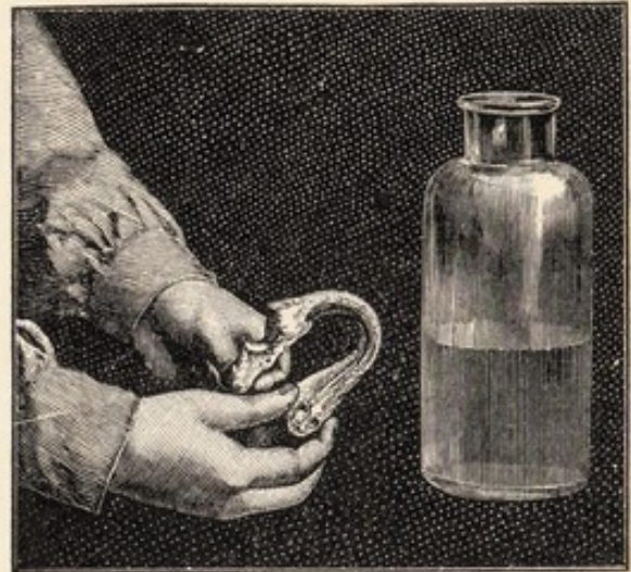
FIG. 7. — Showing how the Small Bone of a Sheep's Leg may be bent after its Earthy Matter has been soaked in an Acid Mixture as described in Experiment
