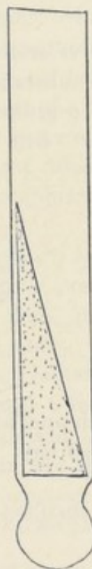
FIG. 211.—Culture tube with bulb to hold glycerine and water below slant of vegetable.
