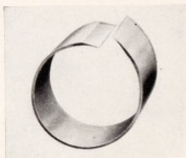
Fig. 44. A wash drawing representing the bending of the band so that the ends overlap. After this is done, the ends are pulled back and sprung one under the other. The tension thus produced will maintain contact during the sweating of the band
