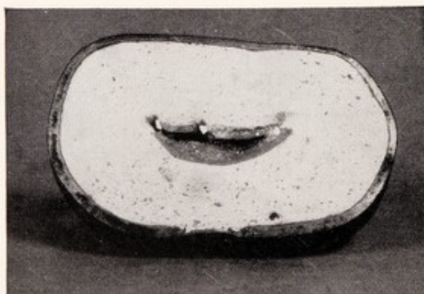
Fig. 492. Platinum boxes and saddle invested in a metal ring preparatory to soldering
