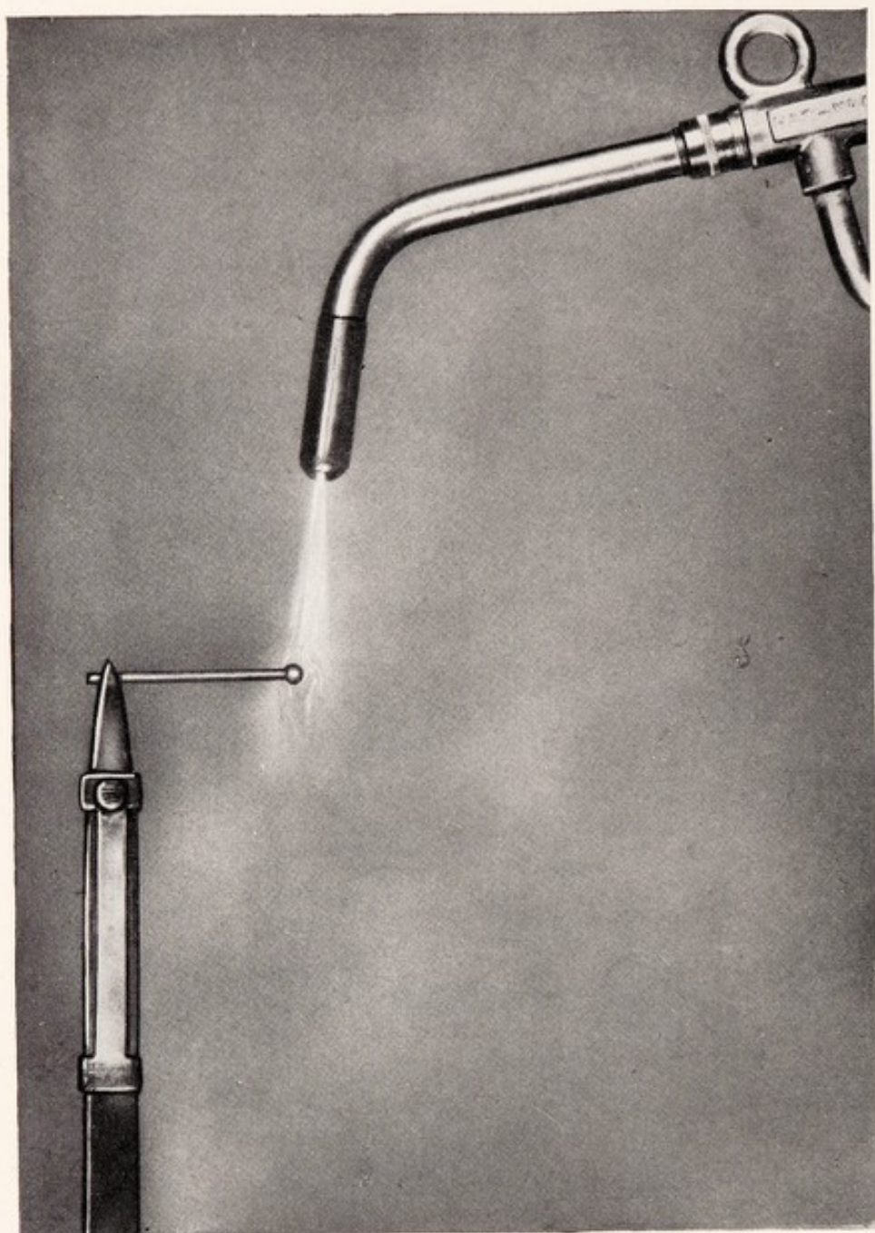
Fig. 346. Fusing ball on the end of wire with blowpipe
