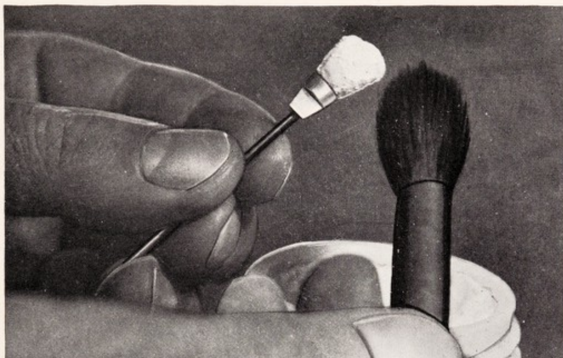
Fig. 148. Excess powdered porcelain is removed with a large, soft, sable brush. This is easily done if the carving was reasonably dry before it was dipped in the powder
