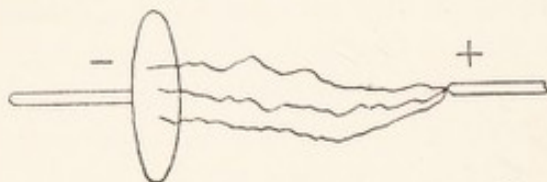
FIG. 36.—Connections of the X-ray tube to the coil, showing the route travelled by the spark when the point is the positive pole and the negative the plate.
