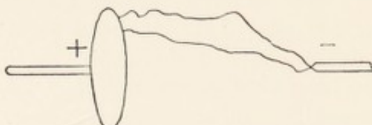
FIG. 11.—Connections of the X-Ray tube to the coil (Schall), showing the appearance when the poles are reversed.
