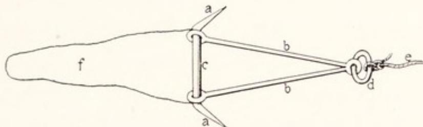
Outlines of Dredge. Upper Figure, Front View; a, a, Blades for Scraping up Material from Bottom with Perforations for Attaching Sack; c, c, Cross Bars; b, b, Arms; d, Rings to which Dredging Rope is Attached
