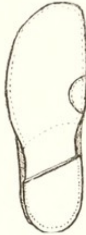
FIG. 2.—Boot with straight inner border, crooked and lengthened heel, patch to thicken sole.
