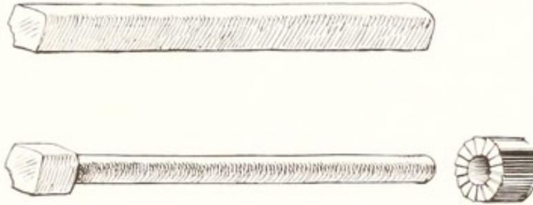
FIG. 168.—The upper drawing represents crest of tibia of the proper cross-section for a hip-fracture peg. The lower drawing illustrates the peg and the author's lathe cutter which was used to shape it.
