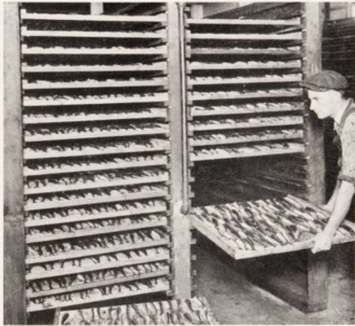
DRYING SARDINES BY ARTIFICIAL HEAT.
