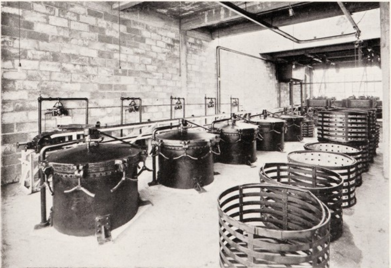
CRATES FOR HOLDING THE CANS AND PERPENDICULAR RETORTS IN WHICH THEY ARE COMMONLY COOKED.
