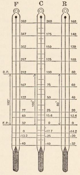
A good idea of the construction of the scales of different thermometers may be obtained by studying the illustration. The zero of the Fahrenheit thermometer is 32 degrees below the zero of other thermometers. It is therefore necessary to subtract 32 from Fahrenheit degrees, before multiplying by the equivalent, when changing to other degrees. And for the same reason, 32 degrees must be added, after multiplying by the equivalent, when changing to Fahrenheit.
