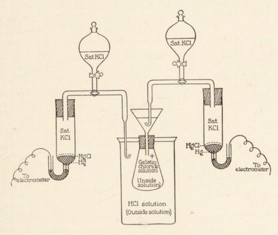
Fig. 40.—Method of measuring the P.D. between gelatin chloride solution in a collodion bag and the outside HCl solution in beaker.
