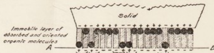
FIG. 24. A diagrammatic representation of the oriented adsorption of organic dipoles at a solid-liquid interface, postulated as a source of the electric double layer.
