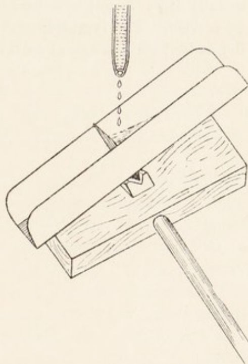
FIG. 80.—Diagram of tilter. The rocking movements are recorded either by allowing the accumulated fluid to actuate a tambour, or by an electro-magnetic signal.
