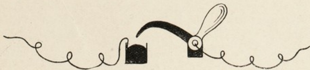
FIG. 9.—Diagram of mercury key.
