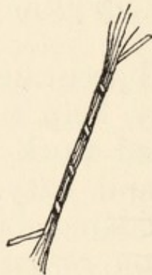
FIG. 2. Silken thread loosely wound round with strip of flat metal.
