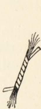
FIG. 1. Silken thread closely wound round with strip of flat metal.
