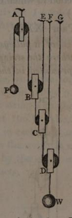
at E; another string is fixed at B, passes under the moveable pulley C, and is fixed at F; &c. in such a manner that the strings are parallel.
