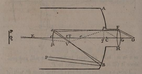
smaller, whose axes are coincident, and whose concave surfaces are turned towards each other; E and e, their centers; T, t, their principal foci, of which, T lies between e and t. In the middle of the larger reflector is an opening, nearly of the same dimensions with the aperture of the smaller, to admit a moveable tube containing a convex eye glass FGH.
