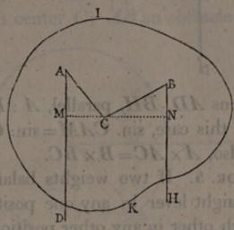
in the directions AD, BH, which coincide with the plane ACB; join AC, CB; then this body may be considered as a lever ACB, and drawing the perpendiculars CM, CN, there will be an equilibrium, when the force acting at A: the force acting at B:: CN: CM\*.
