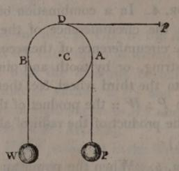
force is exerted at D in the direction DAP, by the power, an equal force is exerted by the weight in the direction DBW; these forces will therefore keep each other in equilibrio.
