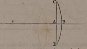
solid generated by the revolution of the figure CD, about the axis rB, is called a *plano-convex lens*.
