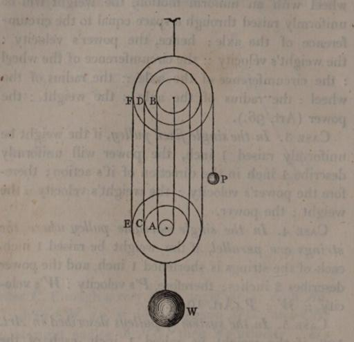
removed to the two centers of motion in the blocks A and B.
