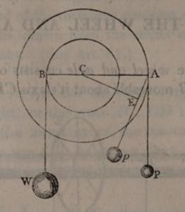
in the same plane, and let CA, CB, be the radii of the wheel and axle, at the extremities of which the power and weight act; then the machine becomes a lever ACB, whose center of motion is C; and since the radii CA, CB, are at right angles to AP and BW, we have P: W:: CB: CA (Art. 82).
