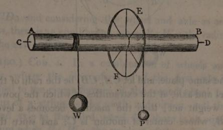
EF so attached to the cylinder that the axis CD passes through it's center, and is perpendicular to it's plane.
