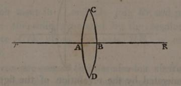
and which meet in C and D; join Rr, and suppose the figure CD to revolve about Rr as an axis; the solid, thus generated, is called a *double convex lens*.
