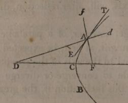
touching the reflector in A; then the angle EAF is equal to the angle DAT, in the ellipse, and to dATin the hyperbola; therefore AD is the reflected ray in the former case, and Ad in the latter; thus D is the focus of reflected rays.
