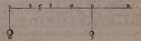
moveable weight P, when placed at E, keep the lever at rest; then when W and P are suspended upon the lever, and the whole remains at rest, W sustains P, and also a weight which would support P when placed at E; therefore  $W \times AC = P \times DC + P \times EC = P \times$ DE; and since AC and P are invariable,  $W \propto ED$ ; the graduation must therefore begin from E; and if P,
