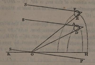
Then the angle ROS, or HOP, measures the altitude of the point S above the horizon; and the altitude
