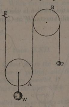
annexed to the center of the pulley A, and the power is applied at P. Then since the strings EA, BA are
