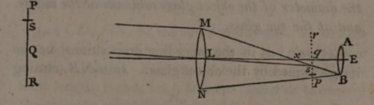
object in S. Then, if x E be greater than q E, all the rays which flow from S, and fall upon MN, will be refracted to the eye glass; for, SM is refracted in the direction MsB; and any other ray of the pencil, as SL, crosses MB at s, and falls somewhere between A
