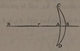
and which meet in C and D; join Rr and produce it to B; the solid generated by the revolution of the figure CD, about the axis RB, is called a *meniscus*.
