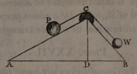
a common altitude CD, by means of a string PCW which passes over the pulley C, and is parallel to the planes, then P: W :: AC : BC.
