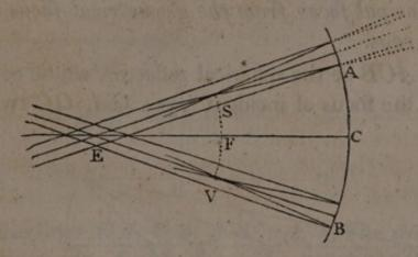
reflector, the foci of reflected rays will lie in the spherical surface SFV, whose center is E and radius EF.
