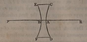
EC, FD parallel to Rr, and equally distant from it; then the solid generated by the revolution of the figure ECDF, about the axis Rr, is called a *double concave* lens.
