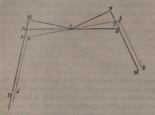
center C, through a very small angle ACa; Join Aa, Bb; draw CM, ax, at right angles to MD; and CN, by, at right angles to NB; then A's velocity : B's velocity :: Ax : By (Art. 148.). Now the triangles Axa, MCA, are similar; because  $\angle xAC = \angle AMC$ +  $\angle MCA$  (Euc. 32. i.) and  $\angle aAC = \angle AMC$ ; therefore,  $\angle xAa = \angle MCA$ ; and the angles at M and x are right angles; consequently, the remaining angles are equal; and
