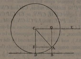
it is to be moved by a force acting in the direction CE; join CA, draw CD perpendicular to the horizon, and from A draw AG, AF, at right angles to CE, CD. Then CA may be considered as a lever whose center of motion is A, CD the direction in which the weight acts, and CE the direction in which the power is applied; and there is an equilibrium on this lever when the power : the weight :: AF : AG.
