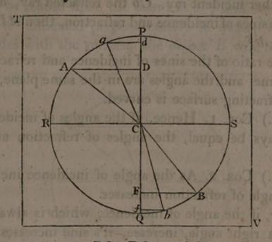
draw the diameters RS, PQ at right angles to each other, and immerse the board into a vessel of water, in such a manner that PQ may be perpendicular to, and RS coincide with the surface of the water. Then, if a ray of light, admitted through a small hole into a dark chamber, be incident upon the surface RS in the direction AC, coincident with the plane of the board, CB, the direction of the refracted ray, is found to coin-
