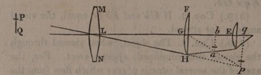
tend to form the image qp, after refraction at the glass FH, form the image ab, between G and q (Art. 223); and this image is viewed through the eye glass E, whose focal length is  $bE^*$ .
