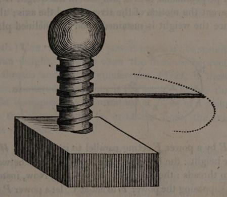
the common axis, by a lever perpendicular to that axis; and a motion will be produced in the direction of the axis, by means of the spiral thread.
