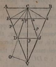
in y, and resolve DC, dC into Dy, yC, dy, yC, of which Dy and dy destroy each other, and 2yC sustains the power. Hence, the power : the sum of the resistances :: 2yC: 2DC :: yC: DC :: sin. CDy or DCA : rad.
