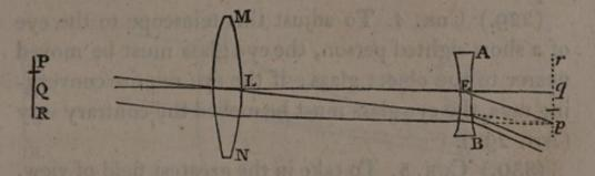
is directed; pqr it's image in the principal focus of the glass L, and therefore in the principal focus of the glass E; then, since the rays tend to form an image in the principal focus of the concave lens E, after refraction at that lens, they will be proper for vision (Art. 290); or, a distinct image of the object PQR, will be formed upon the retina of a common eye.
