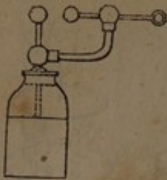
Fig. 124. Medical Jars mounted with Lanes's discharging Electrometer, from 10s. 6d.
