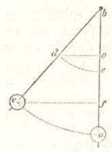
If a pendulum b a be twice as long as another b e, it has twice as much to fall in its descending arc c a, as the other in its arc d e, while in corresponding parts of the two paths, the slope or inclination is always equal.
