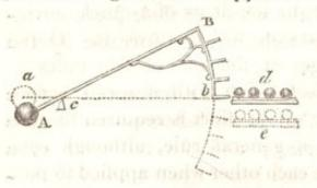
pounds at the end of the rod or lever A B, turning on C as its axis, or fulcrum, and having the arm C B four times as long as the arm CA: one pound at the end
