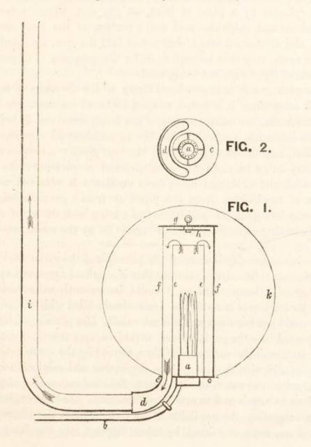
by the small metal ring or knob at the top; i, is the metallic tube chimney; k, a ground globe, which may be applied to the lamp, and which has no opening, except the hole at the bottom, where it rests on the glass-holder; but any other form, as a lotus glass or vase, may be substituted at pleasure.
