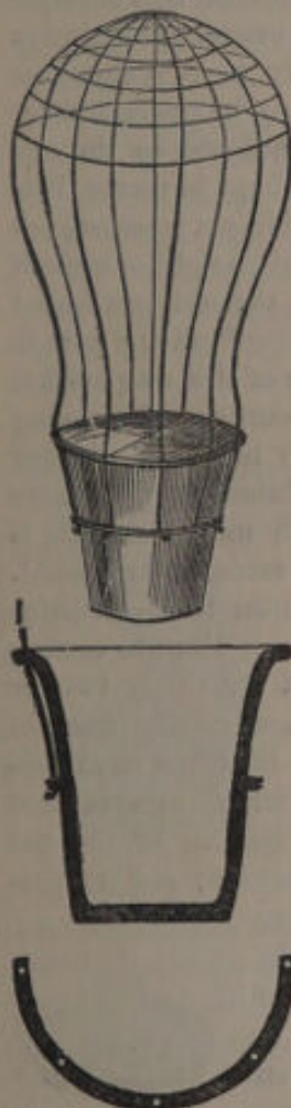
Fig. 57. Pot with pierced rims and bands for introducing wirework.
