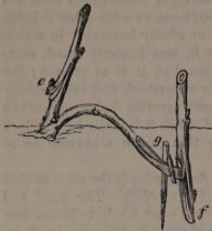
Fig. 184. Layering with the tongue made in the upper side of the shoot.
