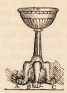
And, generally, if we draw lines joining the extreme points where a body is in contact with the plane on which it rests, the area included within these lines is virtually the base of the body, and there will be an equilibrium, if the vertical through the centre of gravity intersect the horizontal plane any where within this area.
