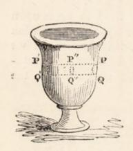
P'Q' represent portions of the sides of such a vessel having the same projection P'Q' upon any given vertical plane; then, from what has been said above, it appears that the horizontal pressures upon these planes perpendicular to the given plane are equal, each, to the pressure of the fluid upon the projection P'Q', and that they are in opposite directions. Since, then, the opposite portions PQ and P'Q' of the sides of the vessel are acted upon
