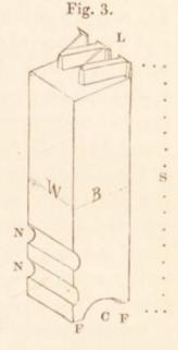
N N. The nicks; these are to show the compositor which is the proper way for the type to stand, and prevents the necessity of looking at every individual letter, for he can feel with his thumb whether he has it the right way upwards; there are sometimes two, three, or four nicks cast in the type, the number and distances of the nicks being intended to distinguish one fount from another.
