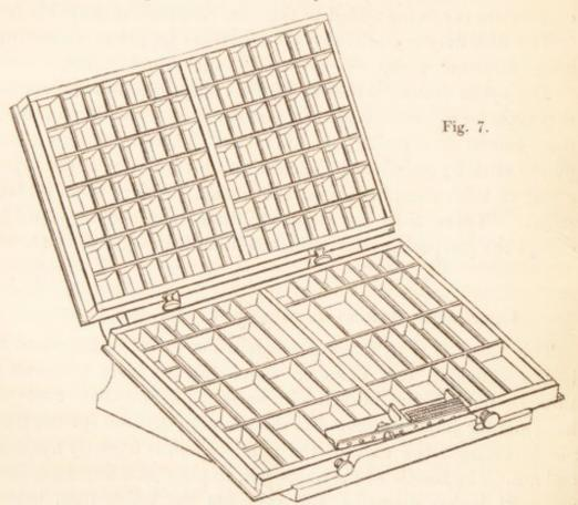
Such an arrangement would however be too cumbersome for most amateurs, and therefore a composing frame is supplied that measures only 20 by 18 inches and 14 inches high. This will support 2 drawers of the large type case at the customary angles, and when placed upon an ordinary table, the height will be found such as to admit of the amateur compositor being seated. Fig. 7 shows the position of the two drawers when placed upon the composing frame ready for operations.
