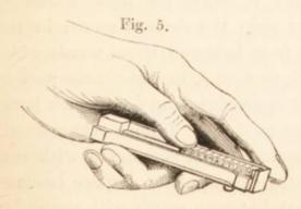
inclination is adopted as in the galley chase, to prevent the types falling. A space line lead should be placed in the composing stick, and all will be then ready for composing, as follows:—
