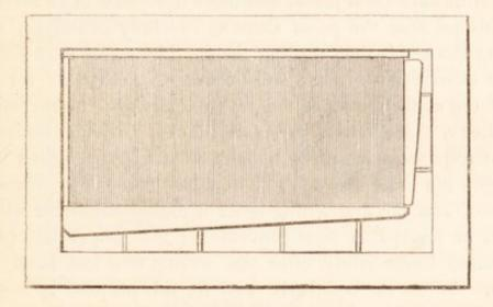
some of the reglets, or some of the wider pieces called furniture, at the ends of the page to extend the length to about 6½ inches. This will leave room for the foot stick which is placed at the bottom of the page, and also for the one or two small wedges called quoins; the side stick is placed at the left hand side of the page, and two quoins are fitted to it, the form is then said to be dressed.
