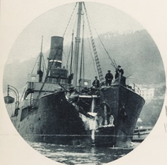
THE LIMERICK STEAMSHIP COMPANY'S "LUIMNEACH" AT DARTMOUTH AFTER HER COLLISION WITH A DESTROYER; SHOWING THE GAFING HOLE IN HER BOW.
