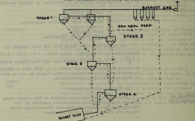
THE SEMI-DRY PROCESS OF CEMENT MANUFACTURE
