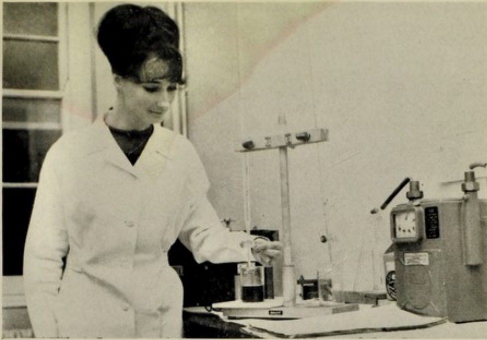
Ascertaining the amount of sulphur oxides collected from the atmosphere in 24 hours by the Smoke and SO 2 Recorder.
