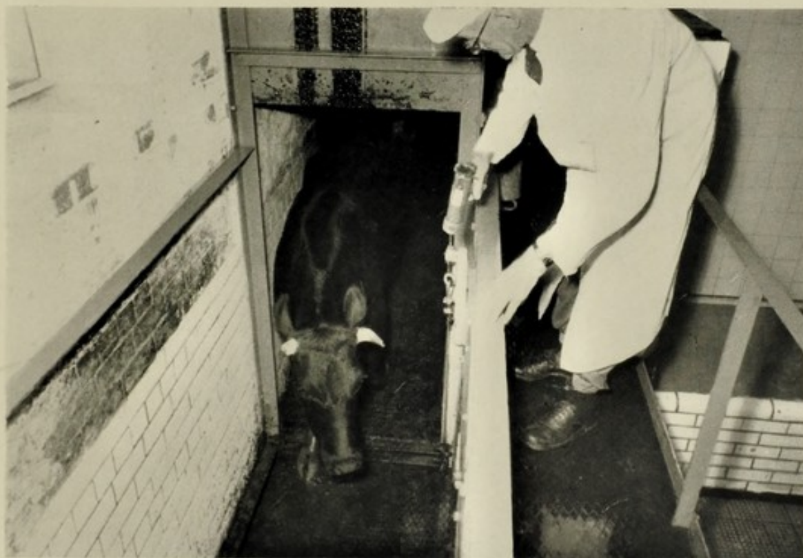
With this modern stunning box the animal walks in unaided, the counter-balanced door is lowered behind it and, after being shot, the carcass is ejected onto the floor.
