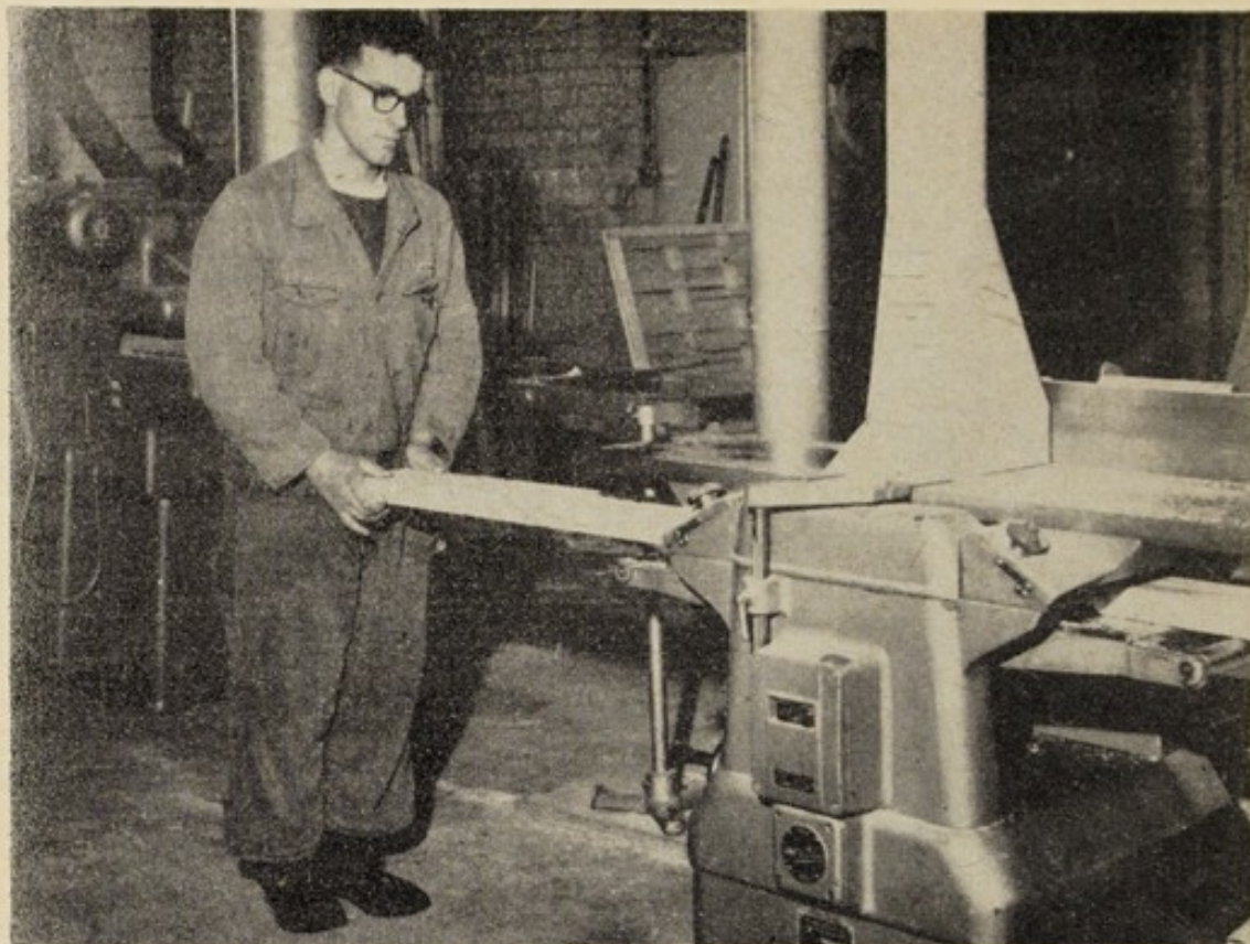
Plate 5/3. The planing machine as installed in the new "factory" with dust extractor fitted.
