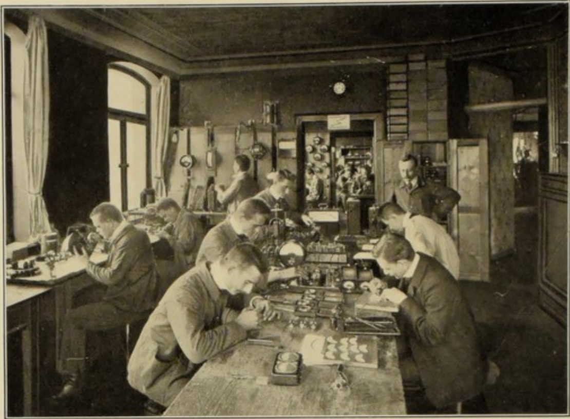
ROOM FOR CALIBRATING GALVANOMETERS.
