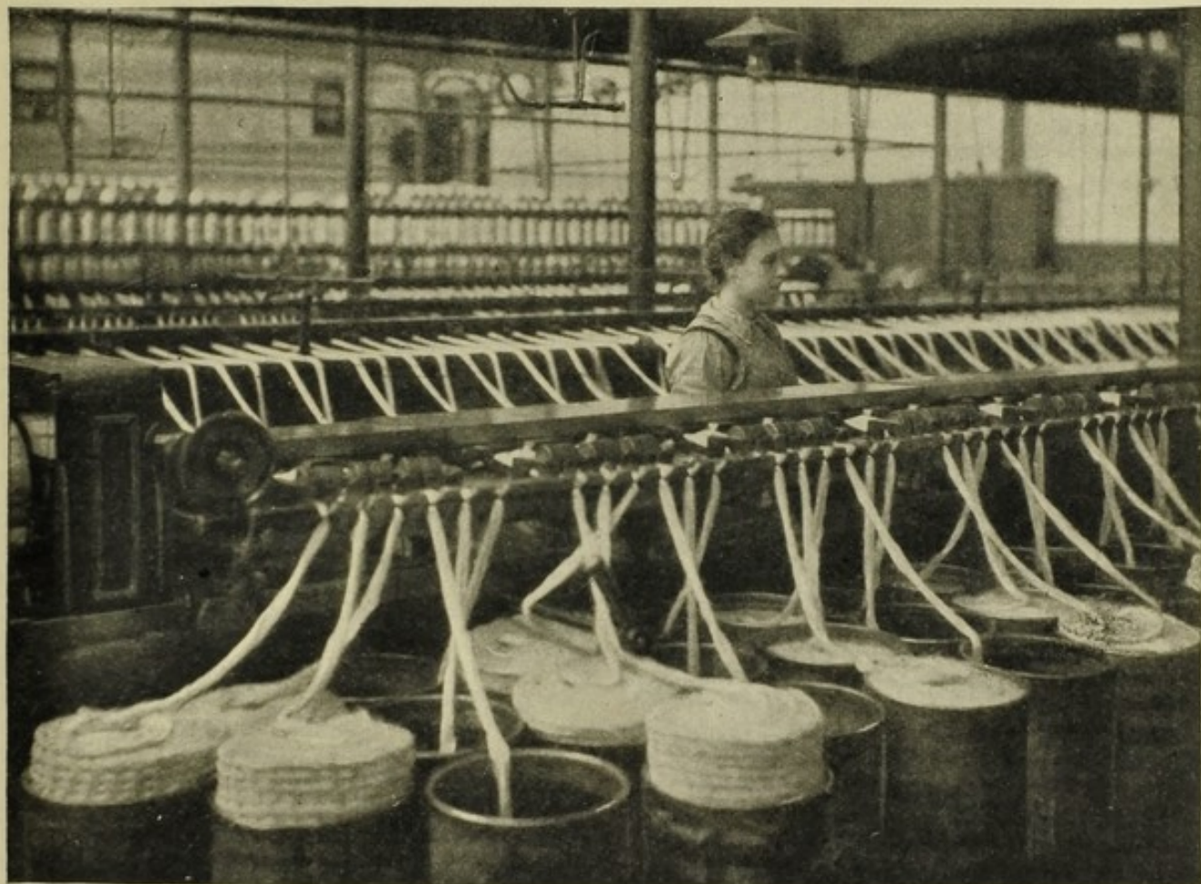
6. SLIVERS PASSING THROUGH A DRAWING-FRAME
