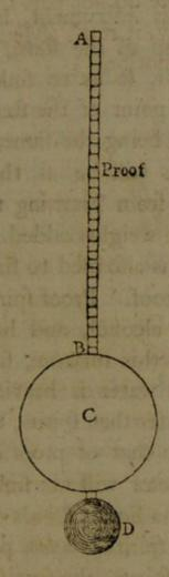
represented by 4000, and each of the divisions by 1 of such parts, and let the whole length of the stem contain 50 of such parts. Now if this instrument be put into one sluid, and it sinks to 30, and in another, it sinks to 20, then the parts immersed will be 3970 and 3980 respectively; and the specific gravities of these two sluids, being inversely as the parts immersed, will be as 3980: 3970. This can only be applied to those sluids which come within the extent of the scale. This instrument
