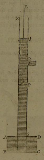
141. Here the fucker Q has no valve, and the air Vol. III. Between
