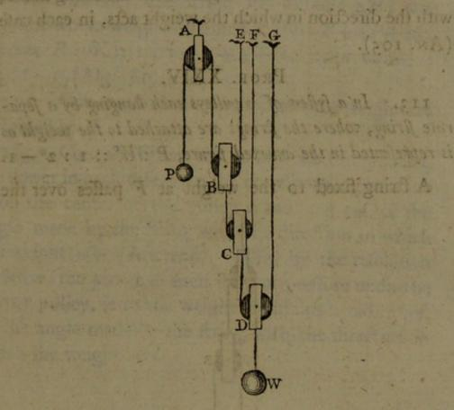
at E; another string is fixed at B, passes under the moveable pulley C, and is fixed at F; &c. in fuch a manner that the strings are parallel.
