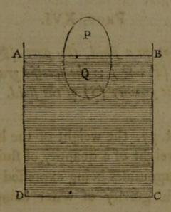
the same pressure supported a quantity of sluid equal in bulk to Q, before the body was immersed, that space being occupied by the sluid; and as the same pressure must sustain the same weight, when there is an equilibrium, the weight of the body must be equal to the weight of a quantity of sluid equal in bulk to Q.
