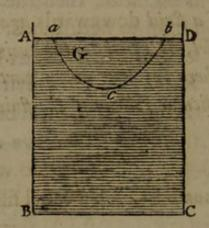
(Mech. Art. 160) just the same as if the whole effect took place at it's center of gravity; therefore the effect of the reaction of the fluid under G must be the same as if it took place at the same point.
