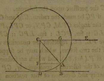
it is to be moved by a force acting in the direction CE; join CA, draw CD perpendicular to the horizon, and from A draw AG, AF, at right angles to CE, CD. Then CA may be confidered as a lever whose center of motion is A, CD the direction in which the weight acts, and CE the direction in which the power is applied; and there is an equilibrium on this lever, when the power: the weight: AF : AG.
