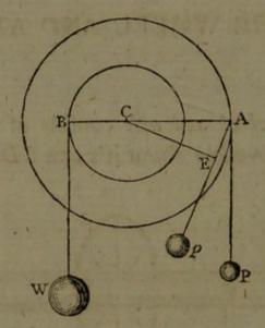
in the same plane, and let CA, CB, be the radii of the wheel and axle, at the extremities of which the power and weight act; then the machine becomes a lever ACB, whose center of motion is C, and since the radii CA, CB, are at right angles to AP and BW, we have P:W::CB:CA (Art. 82).
