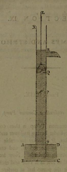
the furface of the water without the pump will force the water a little way up the pump. Now when 2 defcends, it will press down the air under it, and that air will shut the valve at P by pressing upon it, but it will open the valve at 2 by preffing under it, and thus fome of the air will escape. Then when 2 ascends again,
