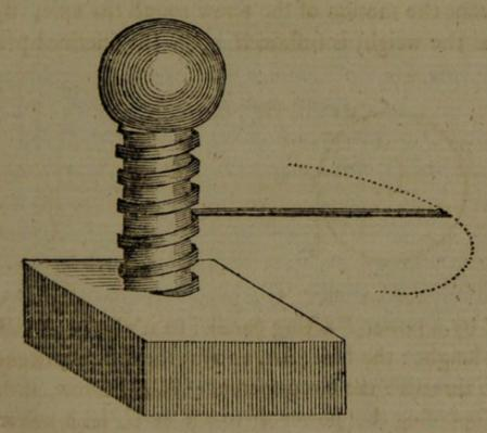
the common axis, by a lever perpendicular to that axis; and a motion will be produced in the direction of the axis, by means of the spiral thread.
