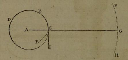
CE by a power F acting parallel to it's base; F:W: the height: the base (Art. 120):: the distance between two threads: the circumference BCD. Now, instead of supposing the power F to act at C, let a power P act perpendicularly at G, on the lever GCA, whose center of motion is A, and let this power produce the same effect at C that F does; then, by the property of
