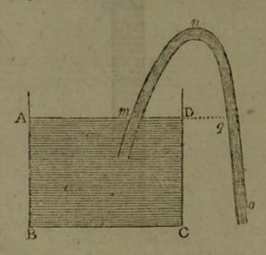
than the surface of the water; then if the air be drawn out, the water will begin and continue to run until
