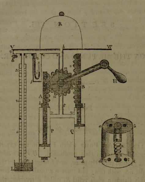
each barrel there is a small hole against which there are two pieces c,d screwed on, containing the valves, each of which is represented by the figure Z, which is a solid piece abcd of brass, through the middle of which there is a cylindrical hole, partly filled with a solid brass cylinder, against the bottom m of which a spiral spring x acts, which rests below against a screw z, by means of which the spring may be rendered stronger or weaker; through the brass there are also
