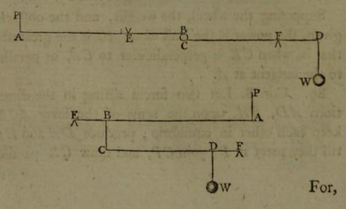
For, the power at A: the weight at B, or C:: EB: EA; and the weight at C: the weight at D:: FD: FC,  $\therefore P: W:: EB \times FD: EA \times FC$ .
