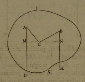
in the directions AD, BH, which coincide with the plane ACB; join AC, CB; then this body may be confidered as a lever ACB, and drawing the perpendiculars CM, CN, there will be an equilibrium, when the force acting at A: the force acting at B:: CN: CM.
