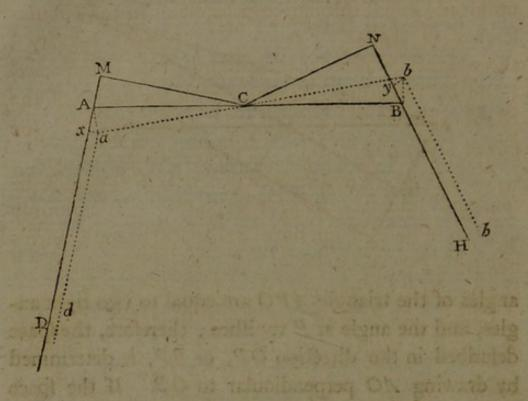
center C, through a very small angle ACa: Join Aa, Bb; draw CM, ax at right angles to MD; and CN, by at right angles to NB; then A's velocity: B's velocity:: Ax: By (Art. 148). Now the triangles Axa, MCA are similar; because  $\angle xAC = \angle AMC + \angle MCA$  (Euc. 32. 1), and  $\angle aAC = \angle AMC$ ; therefore,  $\angle xAa = \angle MCA$ ; and the angles at M and x are right angles; consequently, the remaining angles are equal; and
