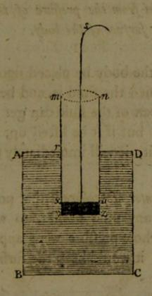
a hollow cylinder, to whose bottom a cylindrical body wxyz, of greater specific gravity than the fluid, may be so closely fitted, that the fluid cannot enter; then
