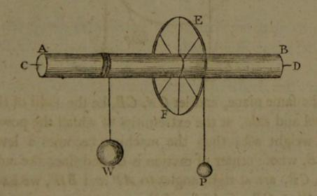
EF so attached to the cylinder that the axis CD passes through it's center, and is perpendicular to it's plane.
