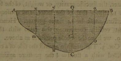
on m perpendicular to that furface is as  $m \times mx$ ; confequently the whole preffure exerted on ACB, in a direction perpendicular to the furface at every point, will be as  $m \times mx + n \times ny + o \times z + &c$ . But (by Mechanics, Art. 172.) if we confider m, n, o, &c. as reprefenting weights in proportion to their respective magnitudes, and the whole area ACB to represent a proportional weight, then  $m \times mx + n \times ny + o \times oz + &c$ .
