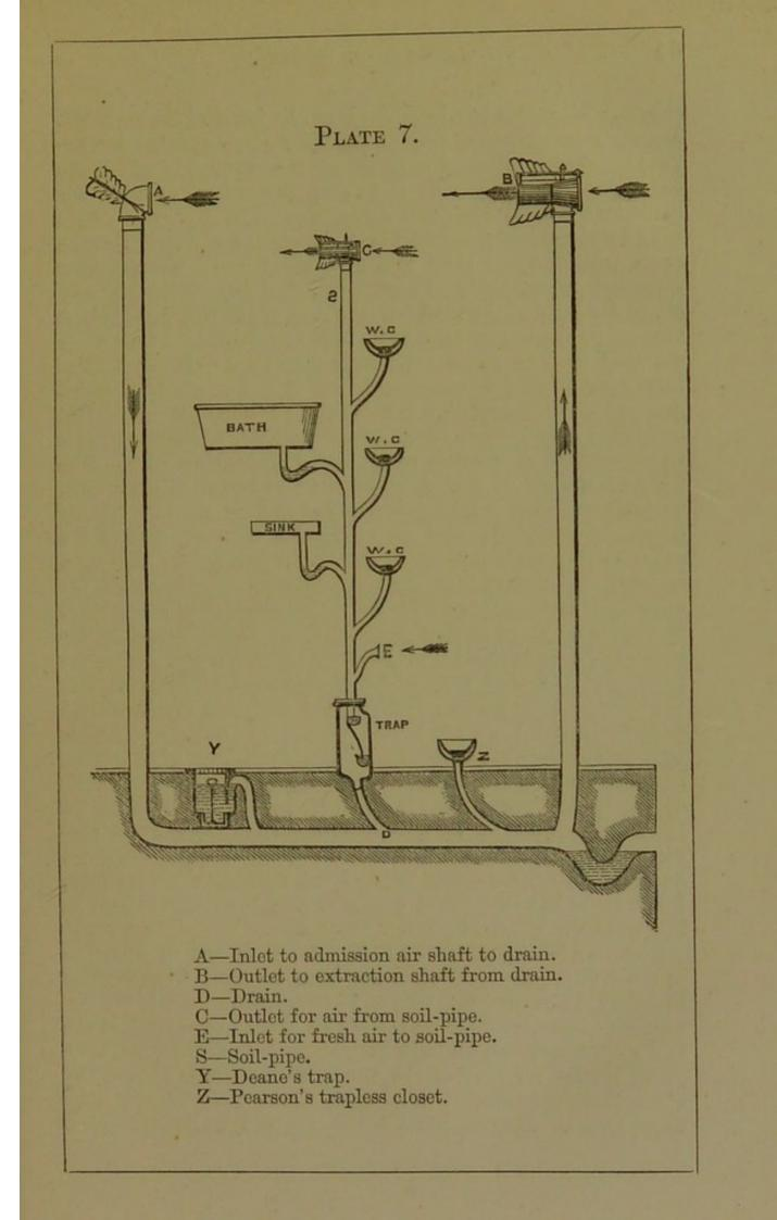
sphere. How this has been done at the hospital through Mr. Banner's intervention may be partially seen from the accompanying sketch intended to illustrate the manner in which the soil-pipes are ventilated, and also the means adopted for securing a free circulation of air in the drains.
