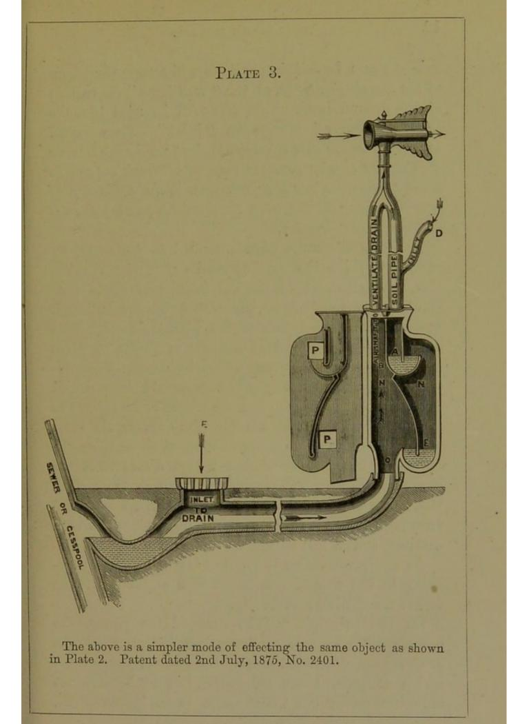
The gases formed in the drain will escape therefrom at the lowest point, viz. at the "ventilator" (so called) at the ground level, unless the cowl be used to make the "ventilator" always an "inlet." From actual experience we are able to certify that with a 4-inch Banner Ventilating Cowl a constant current of fresh air can be made to course along a HORIZONTAL drain a distance of over one thousand feet while the sewage is passing down it in the opposite direction.
