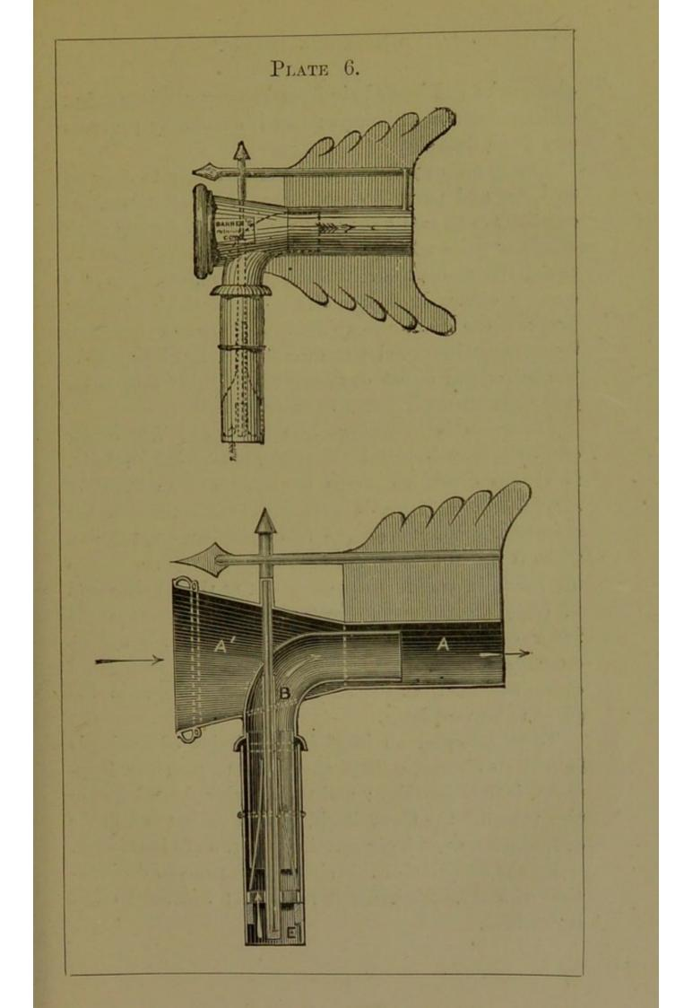
also smoke and heated air from railway carriages, &c., and smoke from chimneys; and it effectually prevents any down draught.
