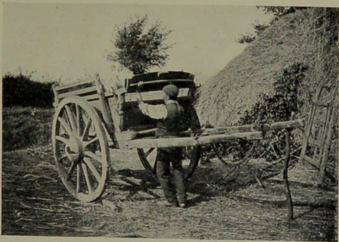
Fig. 2.—Head-board being fixed to front of cart frame after removal of cope and ladder.
