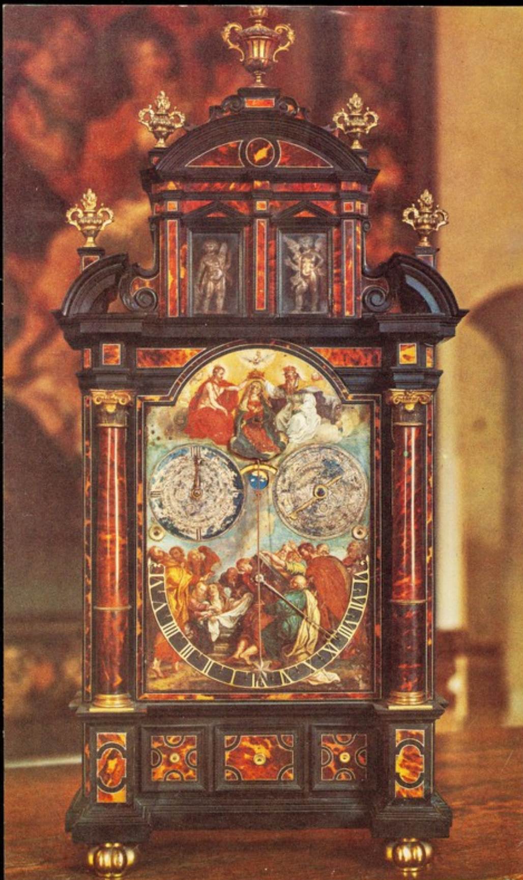
SUN AND MOON CLOCK CIRCA 1680. The chapter ring is marked for twelve hours commencing at VI, through to XII, on again to VI, then returning, and so on. The left dial is the moon dial, with quarters. The right dial has a calendar, months and days, with the signs of the Zodiac. The upper scene depicts the Coronation of the Virgin Mary. Her figure is fixed to the pendulum rod and swings to and fro.
