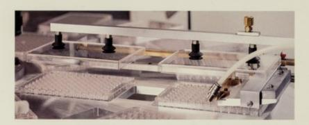
A CCD camera with a field of view 30mm x 40mm is fixed in a stationary position looking down at a colony plate. As each area of the plate is presented to the camera by an x-y table,
