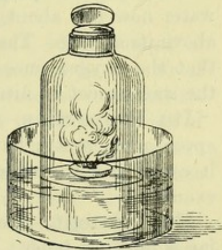
Fig. 4.—Experiment for removing the Oxygen contained in a jar of ordinary atmospheric air.
