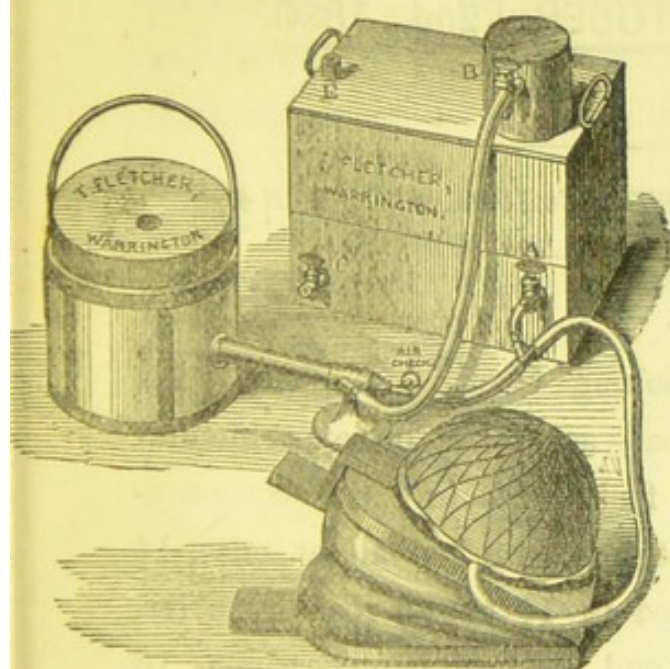
Crucible Furnace for Gas or Petroleum Vapour, showing Gas making attachment in use.
