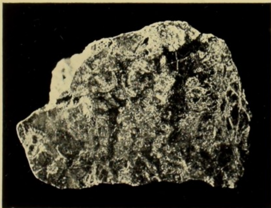
FIG. 3. Sir William Crookes' Pictures of Pitchblende. The lower figure is a daylight photograph. The upper was imprinted in the dark by the rays from the substance.
