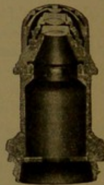
FIG. 12. Objective 1/12, Homogeneous Immersion (Leitz).
