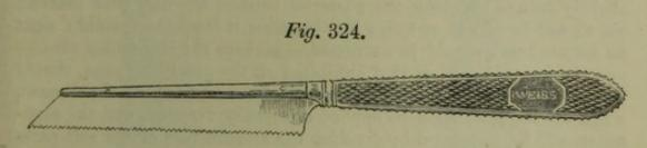
A similar instrument has been advantageously used by Dr. Warren in many of his operations; and, to one accustomed to cut with such tools, there is no difficulty in notching the bone in the manner directed. The handle is about three inches and a half long, the blade the same, and may be a quarter, a half, or a whole inch in depth. A back is required, as the plate is very thin, on purpose to permit the teeth being twisted outwards as in a properly-set saw.
