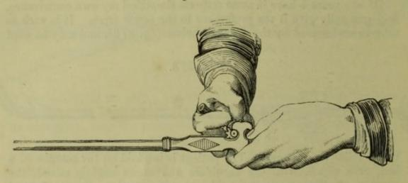
he had yet seen " for crushing the stone; and the figure (373) on the preceding page has been represented by Civiale, in his latest work on lithotrity (1847,) as the "most simple" with which he is acquainted. Mr. Weiss has made some slight changes in this, having placed the rack below again, where I originally had it, with a little modification of the handle and the place for its reception. The French
