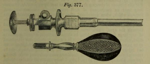
could be made to revolve in such a way that the handle could be applied with perfect ease in whatever position the instrument might lie.
